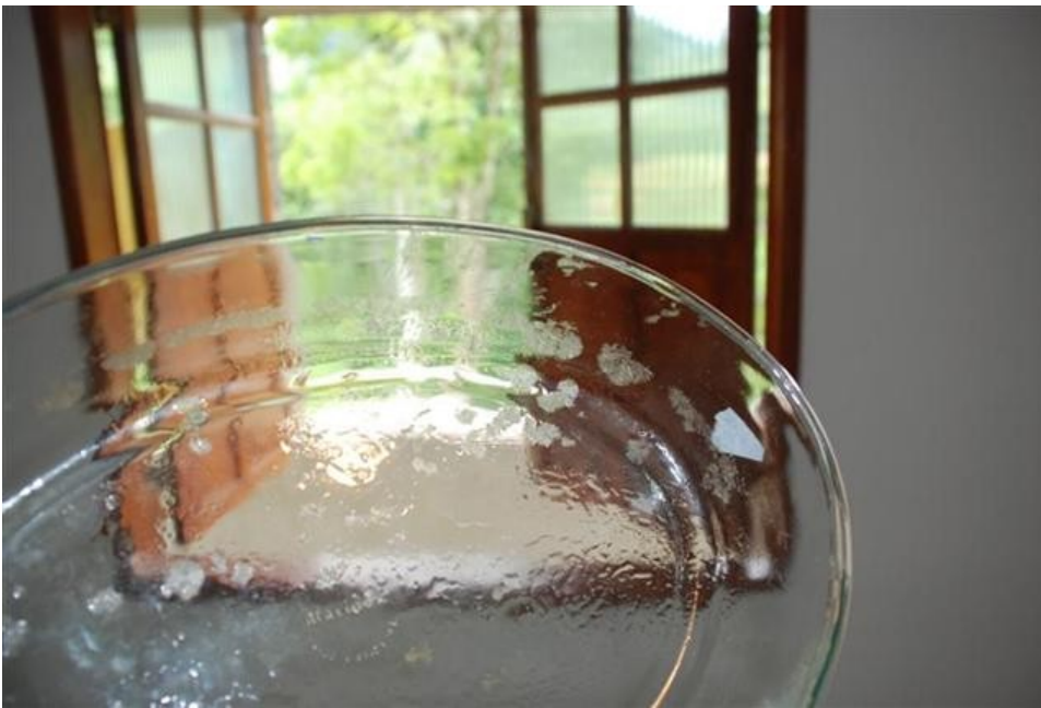
Crystals stuck to glass after freeze precipitation. Notice the white colour, showing high purity of the crystals.
