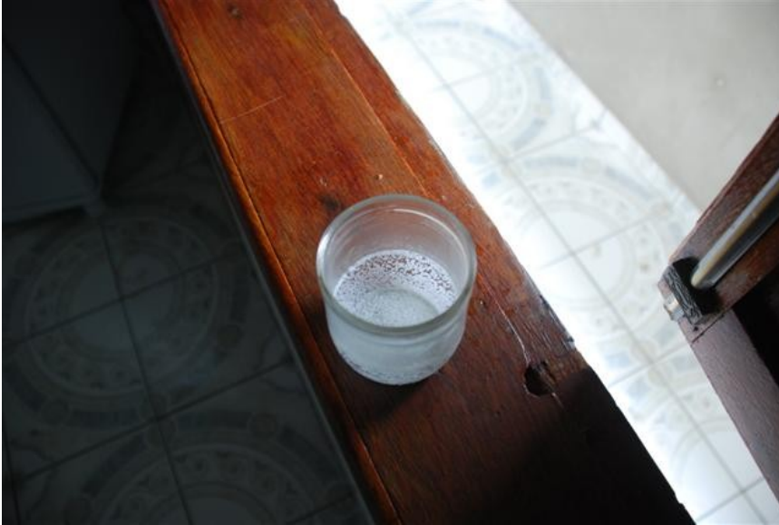
Crystals stuck to glass after freeze precipitation. Notice the white colour, showing high purity of the crystals.
